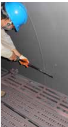
Spark testing of finished top coat of ChemLine® 784/32 (grey colour)
