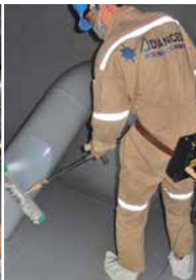
Spark testing of finished top coat of ChemLine® 784/32 (grey colour)
