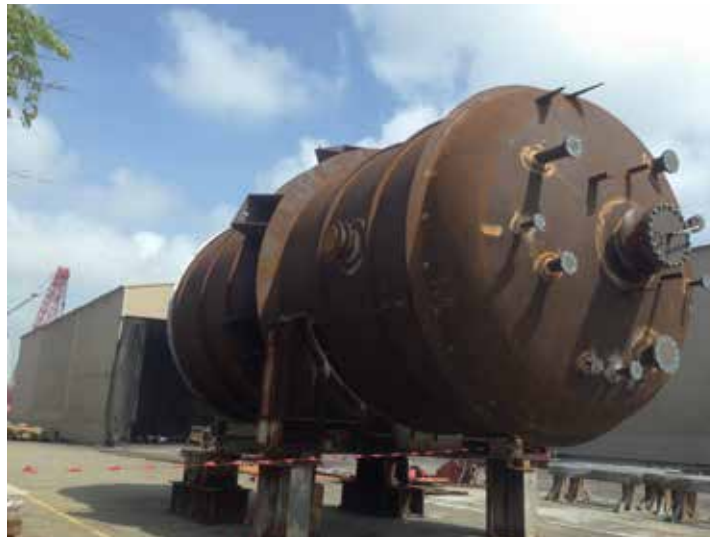
New carbon steel vessel waiting for lining with ChemLine® 784/32 system at the KFPC facility in Taiwan
