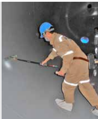
Spark testing of finished top coat of ChemLine® 784/32 (grey colour)
