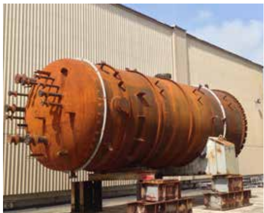
A total of four vessels are ready to be lined with ChemLine® 784/32
