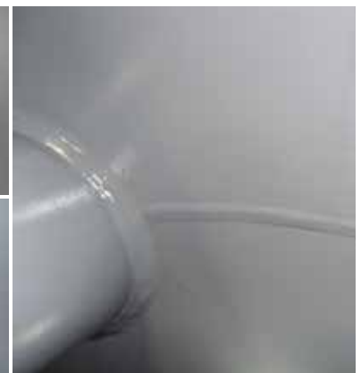
Close up views of the smooth surface of ChemLine® 784/32 coating at a total combined thickness of 12-14 mils
