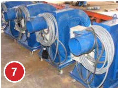
**Photo 7** shows the multiple fans used in each tank. The operator has placed a number of thermocouples within the tank
