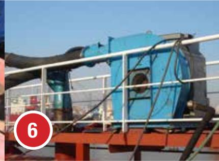
**Photo 6** that forces hot air down into the cargo tank where it is circulated.
