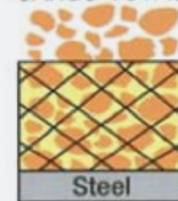
Swelling due to absorption (1)
