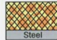
Epoxy with absorbed cargo (2)
