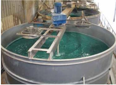
(Left, top and below) As seen here, severe corrosion issues were encountered due to reactions with Zinc Sulphate at high temperatures in these tanks. (Right, top and below) The ChemLine® coating applied internally in the tanks, rectified the corrosion problem. This photo is after four months of the ChemLine® coating in service, with no problems.
