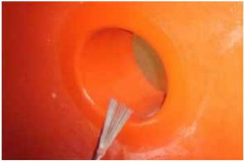
Tanks at this tank terminal storage facility in Barranquilla, located on the north coast of Colombia, required special lining protection to handle corrosive Sulphuric Acid LEFT: Monómeros Colombo Venezolanos' facility in Colombia. RIGHT: Prior to being put into service, the ChemLine® coating in the tank is spark tested as part of a thorough inspection process.
