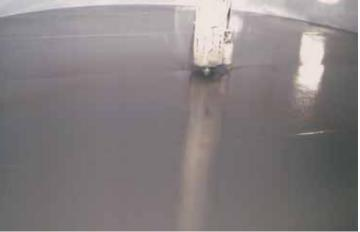
A wine and spirits producer had problems with corrosion in stainless steel and carbon processing and storage tanks. ChemLine® EF was used for corrosion protection and to ensure the lining did not impart any taste or odor to the contents LEFT: Severe tank corrosion issues. RIGHT: ChemLine® as applied solved all problems.
