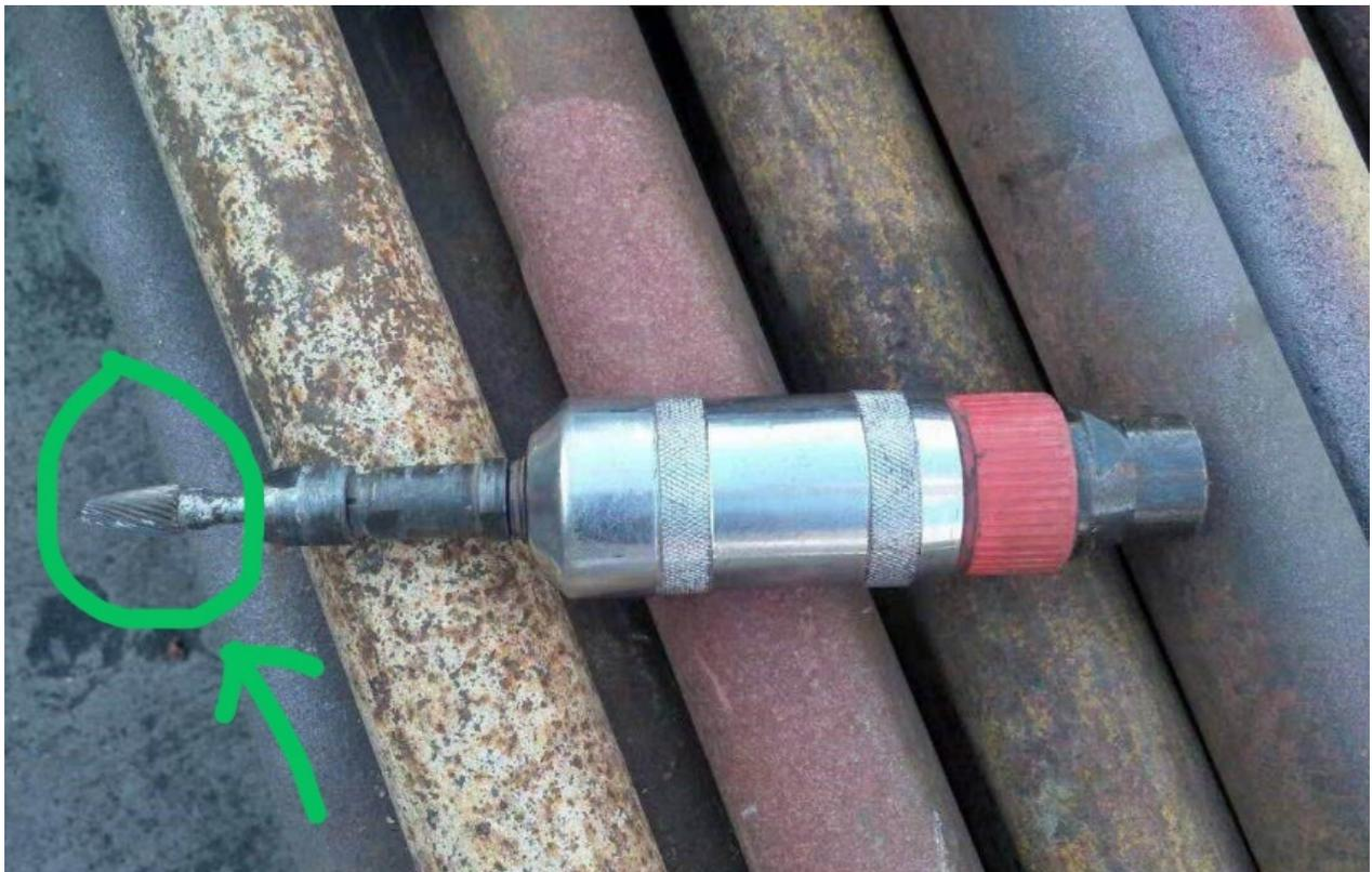
The above photo is the recommended grinding tools for the pinpoint rust area, this grinding head can make some steel profile while not enlarging the bare steel area.
